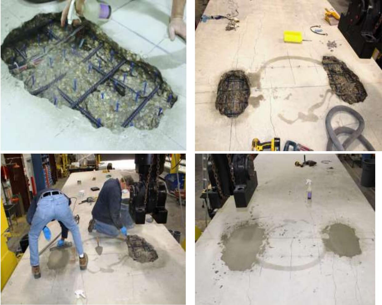
**Figure 4-69 Repair of punching shear damage from Tests C and D.**
