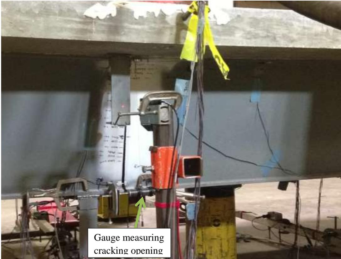
Figure 4-10 Crack opening measuring gauge on the exterior face.
