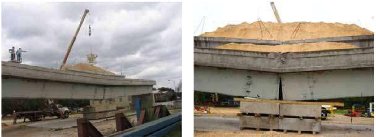
**Figure 1-5 FSEL third bridge fracture test (Source: FHWA Report No FHWA/TX-10/9-5498-1).**
