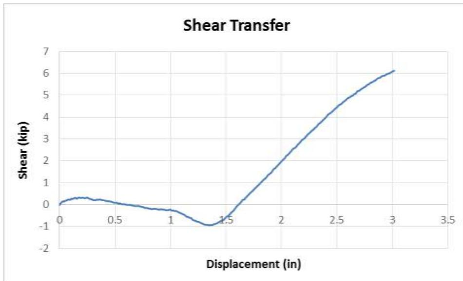
Figure 4-75 Shear transferred through a cross-frame in Test E.
