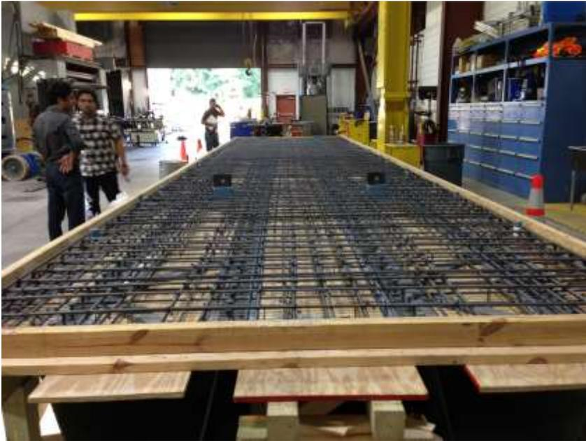
**Figure 3-8 Complete specimen ready for casting.**
