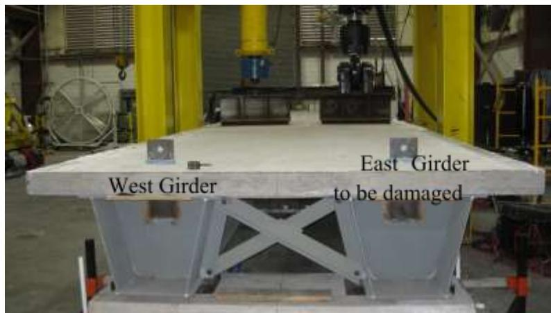
Figure 3-22 Specimen with complete loading setup.
