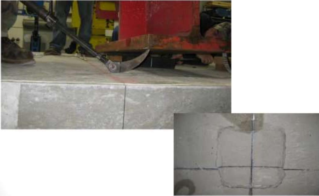
Figure 4-49 Punching damage in test C.
