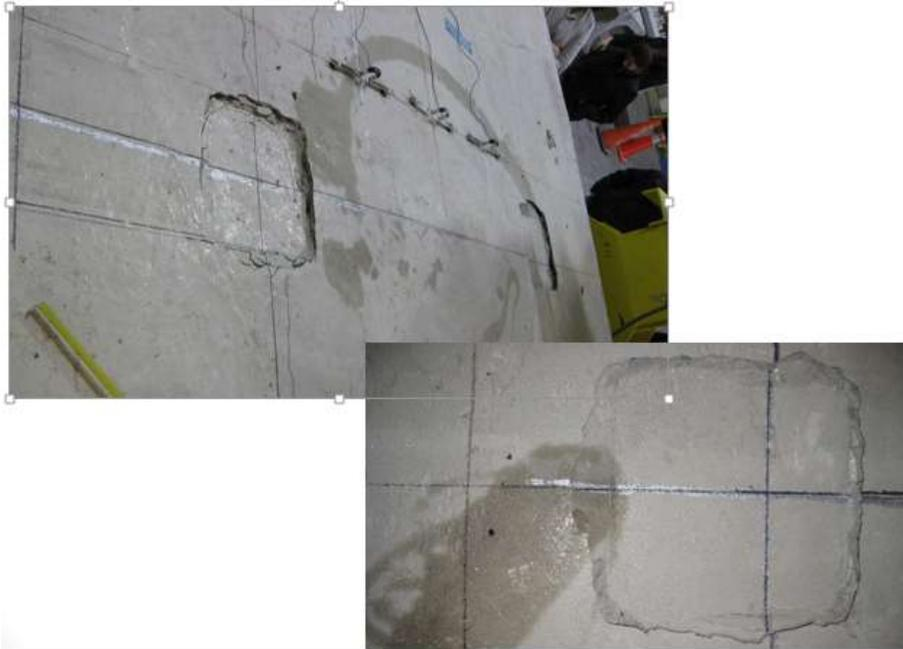
Figure 4-60 Punching damage in Test C.
