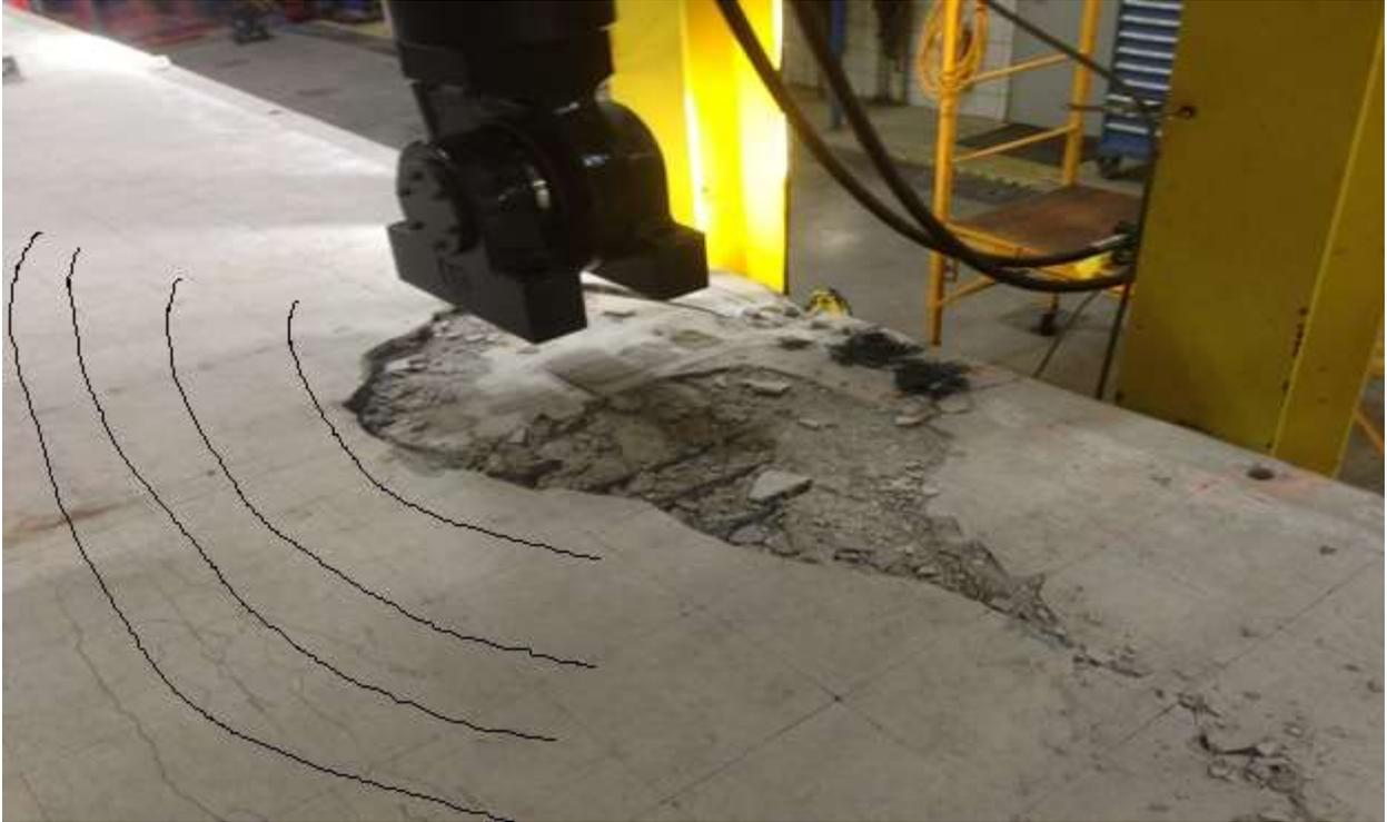
**Figure 4-19 Punching in the top of the concrete surface looking to South.**
