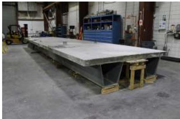
**Figure 4-35 The reconstructed specimen before (left) and after casting (right).**
