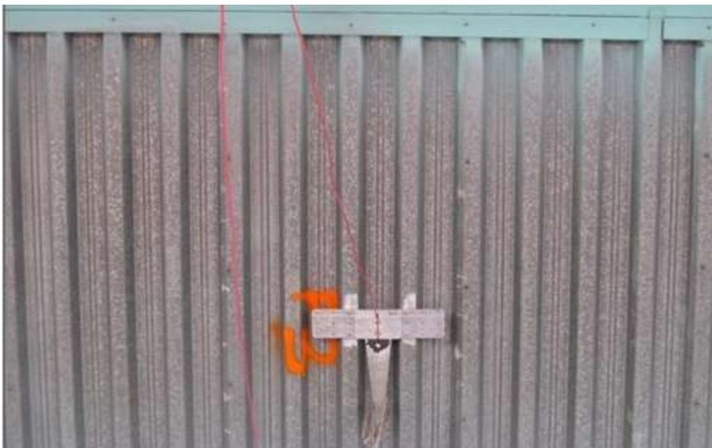
**Figure 7-10 Displacement sensor on SIP form below concrete deck.**
