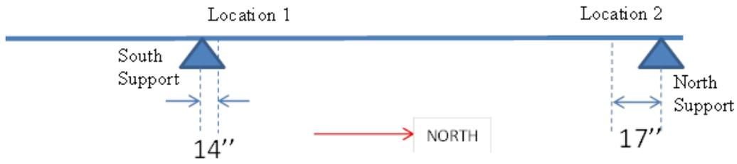
Figure 4-22 Location of potentiometers at supports.
