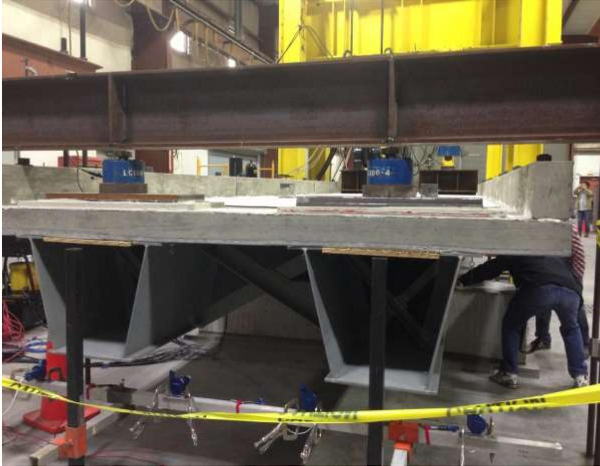
**Figure 3-20 Setup for continuity effect.**
